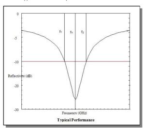
The performance of ECCOSORB® DSF is defined by reflectivity at a single frequency. A generalized performance curve is shown above. The design frequency f0, has a  $\pm 5\%$  bandwidth, designated as f1 and f2.
