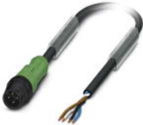
Sensor/Actuator cable, 4-position, PUR halogen-free, Black-gray RAL 7021, Plug straight M12, A-coded, on Free cable end, Cable length: 1.5 m, with plastic knurl
