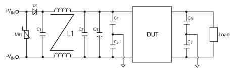
It is recommended to add UR1, D1 and C1 in railway application. C1, L1, C2 and C3 can be modified for required EMI standards. To meet EN61000-4-2, module case should be earth grounded. We offer independent case pin option on request, the location is upon pin 1.
